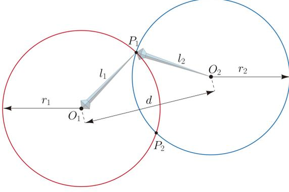
Figure 3: Inverse kinematics as circle-circle intersection
